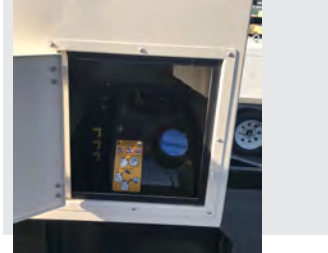
DEF Tank Location
